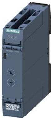
Timing relay, electronic OFF delay without control signal or smooth passing make contact non-volatile 7 time ranges 0.05...600 s 12-240 V AC/DC, 1 change-over contact at 50/60 Hz AC with LED, Screw terminal
