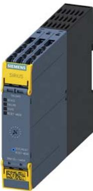
Fail-safe reversing starter, 3RM1, 500 V, 0.55 - 3 kW, 1.6 - 7 A, 24 V DC, screw terminals
