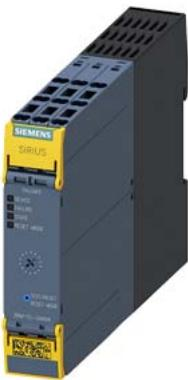
fail-safe direct-on-line starter, 3RM1, 500 V, 0 - 0.12 kW, 0.1 - 0.5 A, 24 V DC, spring-loaded terminal (push-in)
