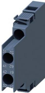
auxiliary switch, lateral, 2 NC, on the left: 31/52, 61/62, on the right: 31/32, 41/42, current path: 1 NC, 1 NC, screw terminal, for contactors 3RT2 and contactor relays 3RH2
