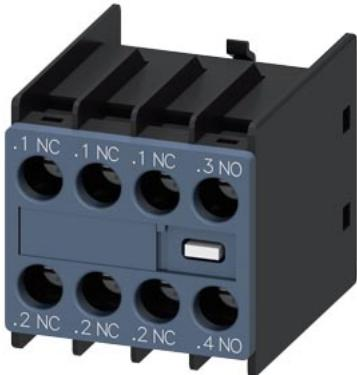
auxiliary switch, on the front, 1 NO + 3 NC, .1/.2, .1/.2, .1/.2, .3/.4, current path: 1 NC, 1 NC, 1 NC, 1 NO, screw terminal, for contactors 3RT2 and contactor relays 3RH2
