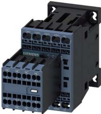
contactor relay, 4 NO + 4 NC, 110 V AC, 50/60 Hz, spring-loaded terminal, frame size S00, removable auxiliary switch
