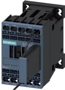
contactor relay railway, 2 NO + 1 NC, 125 V DC, 0.7-1.25\*Us, with integrated suppressor diode, spring-loaded terminal, frame size S00, DIN-rail mounting optimized for transport (20 G)
