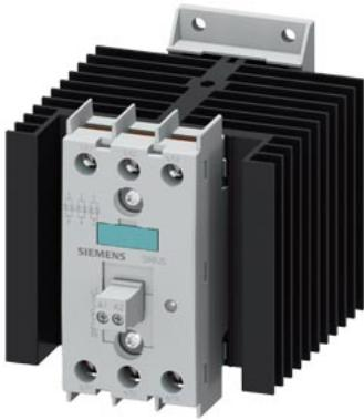
Solid-state contactor 3-phase 3RF2 AC 51 / 30 A / 40 °C 48-600 V / 4-30 V DC 3-phase controlled screw terminal Blocking voltage 1200 V
