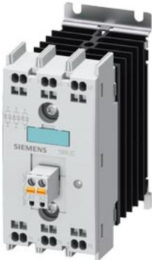
Solid-state contactor 3-phase 3RF2 AC 51 / 10 A / 40 °C 48-600 V / 4-30 V DC 3-phase controlled Spring-type terminal Blocking voltage 1200 V
