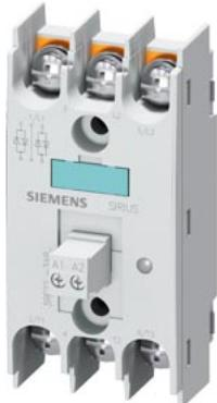
semiconductor relay, 3-phase 3RF2 55 A / 40 °C 48-600 V / 4-30 V DC 2-phase controlled ring cable terminal blocking voltage 1200 V for mounting on available cooling surfaces
