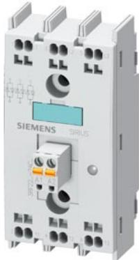
semiconductor relay, 3-phase 3RF2 55 A / 40 °C 48-600 V / 4-30 V DC 3-phase controlled spring-loaded terminal blocking voltage 1200 V for mounting on available cooling surfaces
