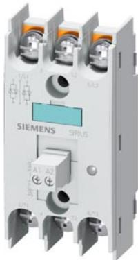
semiconductor relay, 3-phase 3RF2 30 A / 40 °C 48-600 V / 4-30 V DC 2-phase controlled ring cable terminal blocking voltage 1200 V for mounting on available cooling surfaces
