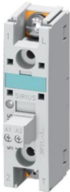
semiconductor relay, 1-phase 3RF2 width 22.5 mm, 20 A 24-230 V / 24 V DC ring cable terminal for mounting on available cooling surfaces
