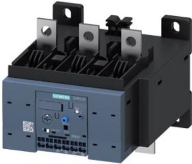
Overload relay 50...200 A for motor protection Size S6, Class 20E Contactor mounting/stand-alone installation Main circuit: busbar connection Auxiliary circuit: Spring-type terminal Manual-Automatic-Reset
