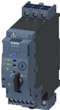
\*\*\*phase-out type\*\*\* compact starter direct-on-line starter for IO-Link 690 V 24 V DC 0.1...0.4 A IP20 connection main circuit: screw terminal connection control circuit: screw terminal alternative 3RK1308 or 3RA8 requirement controller such as ET 200SP in use
