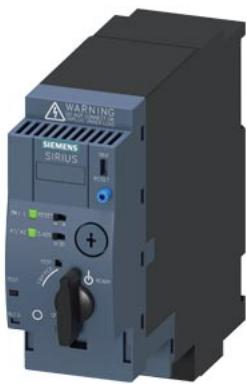
SIRIUS Compact load feeder DOL starter 690 V 110...240 V AC/DC 50...60 Hz 0.32...1.25 A IP20 Connection main circuit: plug-in, without terminals Connection auxiliary circuit: plug-in, without terminals
