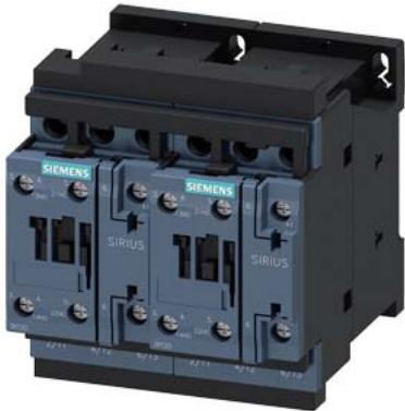
reversing contactor assembly, AC-3e/AC-3, 17 A, 7.5 kW / 400 V, 3-pole, 110 V AC, 50 Hz / 120 V, 60 Hz, screw terminal, electrical and mechanical interlock, auxiliary contacts: 2 x 1 NO
