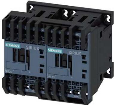
reversing contactor assembly, AC-3e/AC-3, 16 A, 7.5 kW / 400 V, 3-pole, 24 V DC, spring-loaded terminal, electrical and mechanical interlock
