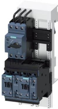
Fuseless motor starter Reversing operation 600VAC Size S0 1.1-1.6A 24V DC screw connection For snapping onto 60 mm busbar systems Type of coordination 2 IQ = 150 KA Also full fills type Of coordination 1 1NO+1NC (per contactor)
