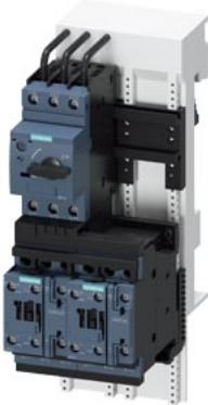
Fuseless motor starter Reversing operation 600VAC Size S0 0.7-1A 110/120VAC 50/60HZ screw connection For snapping onto 60 mm busbar systems Type of coordination 2 IQ = 150 KA Also full fills type Of coordination 1 1NO+1NC (per contactor)
