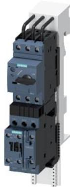
Fuseless motor starter Direct start 600VAC Size S0 1.1-1.6A 220/240VAC 50/60HZ screw connection For snapping onto 60 mm busbar systems Type of coordination 2 IQ = 150 KA Also full fills type Of coordination 1 1NO+1NC (contactor)
