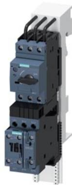
Fuseless motor starter Direct start 600VAC Size S0 0.55-0.8A 24V DC screw connection For snapping onto 60 mm busbar systems Type of coordination 2 IQ = 150 KA Also full fills type Of coordination 1 1NO+1NC (contactor)
