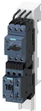
Fuseless motor starter Direct start 600VAC Size S0 0.55-0.8A 110/120VAC 50/60HZ screw connection For snapping onto 60 mm busbar systems Type of coordination 2 IQ = 150 KA Also full fills type Of coordination 1 1NO+1NC (contactor)
