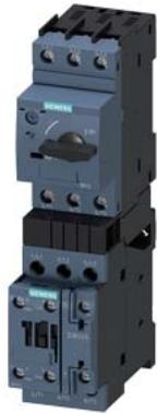
Fuseless motor starter Direct start 600VAC Size S0 0.55-0.8A 110/120VAC 50/60HZ screw connection For screw mounting Or 35 mm rail-mounting Type of coordination 2 IQ = 150 KA Also full fills type Of coordination 1 1NO+1NC (contactor)
