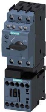
Load feeder fuseless, Direct-on-line starting 400 V AC, Size S00 4.50...6.30 A 24 V DC screw terminal for installation on standard mounting rail (also fulfills type of coordination 1) Type of coordination 2,  $I_q = 150 \text{ kA}$  1 NC (contactor) 1 NO+1 NC (circuit breaker, transverse)
