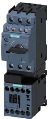
Fuseless motor starter Direct start 600VAC Size S00 2.2-3.2A 24V DC screw connection For screw mounting Or 35 mm rail-mounting Type of coordination 2 IQ = 150 KA Also full fills type Of coordination 1 1NO+1NC (MSP) 1NO (contactor)
