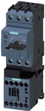
Load feeder fuseless, Direct-on-line starting 400 V AC, Size S00 3.50...5.00 A 230 V AC screw terminal for installation on standard mounting rail Type of coordination 1,  $I_q = 150$  kA 1 NO (contactor)
