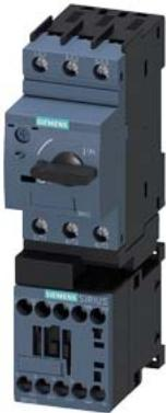
Load feeder fuseless, Direct-on-line starting 400 V AC, Size S00 2.20...3.20 A 24 V DC screw terminal for installation on standard mounting rail (also fulfills type of coordination 1) Type of coordination 2,  $I_q = 150 \text{ kA}$  1 NO (contactor) with diode (integrated)
