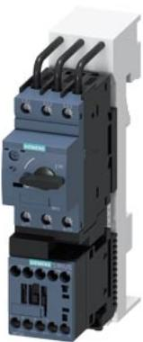
Load feeder fuseless, Direct-on-line starting 400 V AC, Size S00 0.90...1.25 A 230 V AC screw terminal for 60 mm busbar systems (also fulfills type of coordination 1)
