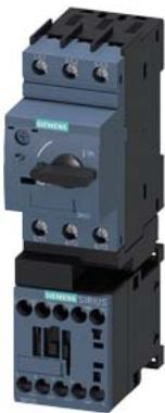
Load feeder fuseless, Direct-on-line starting 400 V AC, Size S00 0.28...0.40 A 230 V AC screw terminal for installation on standard mounting rail (also fulfills type of coordination 1) Type of coordination 2,  $I_q = 150 \text{ kA}$  1 NO (contactor)
