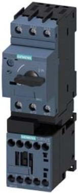
Load feeder fuseless, Direct-on-line starting 400 V AC, Size S00 0.18...0.25 A 24 V DC screw terminal for installation on standard mounting rail (also fulfills type of coordination 1) Type of coordination 2,  $I_q = 150 \text{ kA}$  1 NO (contactor)
