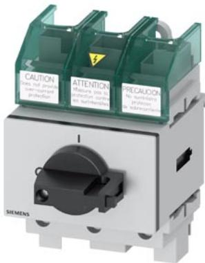
SENTRON 3LD5 switch disconnector UL, main switch, 3-pole, approved according to UL 489, UL 60947-4-1 and IEC 60947-3, UL: 60 A, SCCR 50 kA at 480 V AC, operational power @ 480 V AC 3-phase: 40 hp, IEC: 63 A, operational power at AC-23 A at 400 V: 30 kW, floor mounting with direct operating mechanism, black including terminal covers for the infeed side for the infeed side
