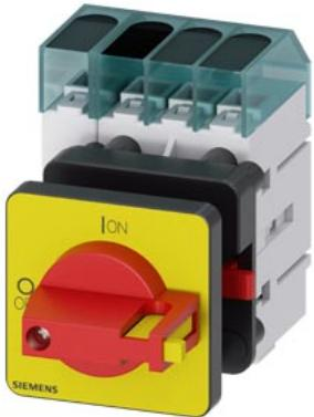
Load disconnector 3LD3, Iu 63 A Main switch 3-pole + N Rated operating capacity at AC-23 A at 400V 22.0 kW Front plate mounting Basic switch with Central hole mounting 22.5mm Toggle drive red / yellow 48x48 mm
