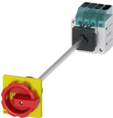
3LD3 switch disconnector, I<sub>u</sub> 63 A main switch 3-pole + N rated operational power at AC-23 A at 400 V 22.0 kW floor mounting basic switch with door coupling center-hole mounting 22.5 mm rotary operating mechanism red/yellow 66 x 66 mm with auxiliary switches 1 NO + 1 NC
