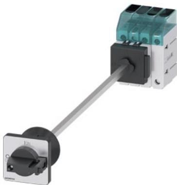
Load disconnector 3LD3, Iu 63 A Main switch 3-pole + N Rated operating capacity at AC-23 A at 400V 22.0 kW floor mounting Basic switch with door coupling Central hole mounting 22.5mm Toggle drive black 48x48 mm
