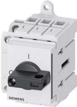
3LD3 switch disconnector, I<sub>u</sub> 40 A main switch 3-pole rated operational power at AC-23 A at 400 V 18.5 kW installation in distribution boards basic switch with knob-operated mechanism black with auxiliary switches 1 NO + 1 NC
