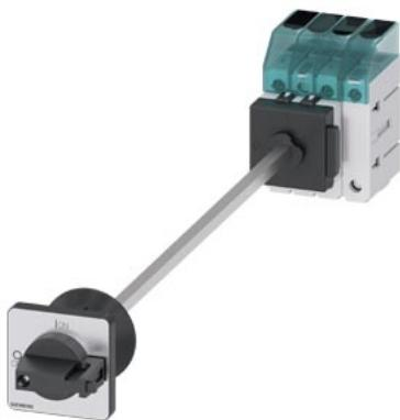
Load disconnector 3LD3, Iu 32 A Main switch 3-pole + N Rated operating capacity for AC-23 A at 400V 11.5kW floor mounting Basic switch with door coupling Central hole mounting 22.5mm Toggle drive black 48x48 mm
