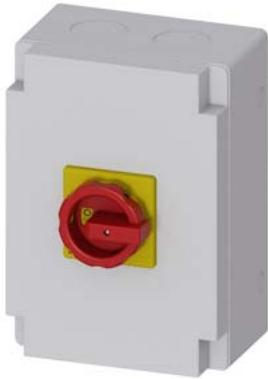
SENTRON, Switch disconnector 3LD, emergency switching-off switch, 3- pole, Iu: 100 A, operating power / at AC-23 A 400 V: 37 kW, Molded plastic encapsulation for inch cable gland, rotary operating mechanism, red/yellow
