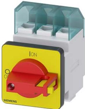
SENTRON, Switch disconnector 3LD, emergency switching-off switch, 3- pole, I<sub>u</sub>: 32 A, operating power / at AC-23 A 400 V: 11.5 kW, front-mounted, knob-operated mechanism, red/yellow, 4-hole mounting of the handle
