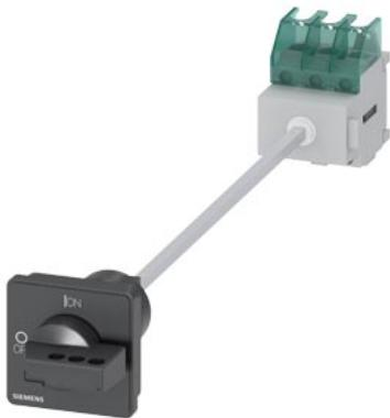
SENTRON, switch disconnector 3LD, main switch, 3-pole,  $I_{u}$ : 32 A, operating power / at AC-23 A at 400 V: 11.5 kW, floor mounting with door coupling, defeatable knob-operated mechanism, black, 4-hole mounting of the handle
