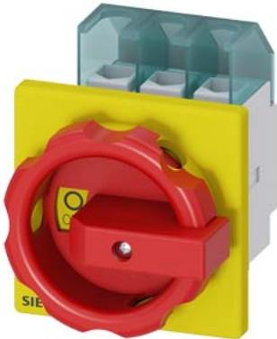
SENTRON, Switch disconnector 3LD, emergency switching-off switch, 3- pole, Iu: 32 A, operating power / at AC-23 A 400 V: 11.5 kW, front-mounted, rotary operating mechanism, Red / yellow, 4-hole mounting of the handle
