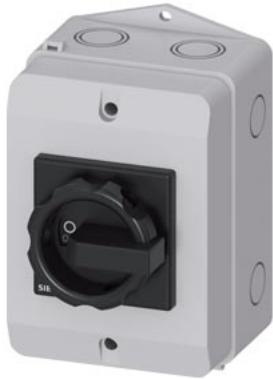
SENTRON, Switch disconnector 3LD, main switch, 3-pole, I<sub>u</sub>: 25 A, Operating power / at AC-23 A at 400 V: 9.5 kW, molded-plastic encapsulation for inch cable gland, 1 NC, 1 NO, rotary operating mechanism, black
