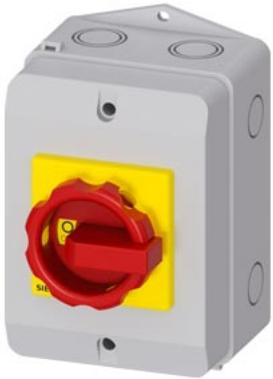
SENTRON, Switch disconnector 3LD, emergency switching-off switch, 4- pole, 16 A, operating power at AC-23 A at 400 V: 7.5 kW, molded-plastic encapsulation for metric cable gland, rotary operating mechanism, red/yellow
