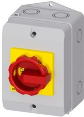
SENTRON, Switch disconnector 3LD, emergency switching-off switch, 3- pole, Iu: 16 A, operating power / at AC-23 A 400 V: 7.5 kW, Molded plastic encapsulation for inch cable gland, 1 NC, 1 NO, rotary operating mechanism, red/yellow
