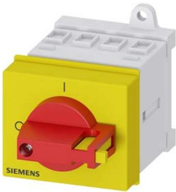
SENTRON, Switch disconnector 3LD, emergency switching-off switch, 4- pole, Iu: 16 A, operating power / at AC-23 A 400 V: 7.5 kW, installation in distribution boards, knob-operated mechanism, Red / yellow, handle direct at the switch
