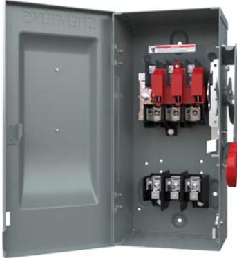
Siemens Low Voltage Circuit Protection Heavy Duty Safety Switches. Type: ENCLOSED, SAFETY SWITCH Std: UL V. Rating: 600V A. Rating: 60A Wattage: 3W No. Of Poles: 3P F. Rating: 60Hz Action: SINGLE THROW Material: STEEL Enclosure: TYPE 1. 2-3 point mounting holes. O. Cycles: 10000 O. Temperature: (-20F-120F) AMBIENT TEMPERATURE Environmental Conditions: INDOOR
