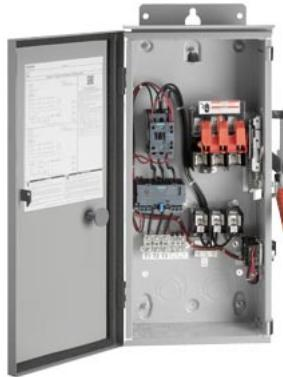
Slim Line Pump Control Panel NEMA size 1 Three phase full voltage Solid-state overload relay OLR amp range 5.5-22A 460VAC 60Hz Coil 30A fusible disconnect 30A/600V fuse clip 1NC / 1NO auxiliary contacts HOA Sel. Sw. <(>&<)> Start/Stop 3-point power terminal block 3-point control terminal block 3-point ground lug Enclosure NEMA type 3/3R Weather proof outdoor use
