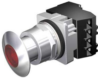
30mm Command/52, Chrome Finish Heavy Duty, Watertight/Oiltight Complete Metal Unit Illuminated Push-Pull Operator Full Voltage, 120V AC/DC LED Lamp Mushroom Head Cap Small 1 3/4" (44.5 mm) Metal, Chrome with Red Lens 2 Position Maintained, Pull-to-Release with 1 N.O. - 1 N.C. Heavy Duty Contacts, A600/P600 UL Listed, CSA Certified NEMA 1,3,3R,4,4X,12,13 & Automotive Standards
