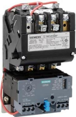
Non-reversing motor starter Size 0 Three phase full voltage Solid-state overload relay OLRelay amp range 3-12A 110-120/220-240VAC 60HZ coil Combination type No enclosure
