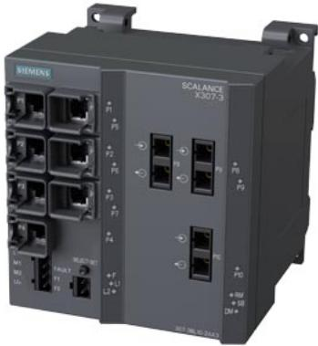
SCALANCE X307-3, managed plus IE switch, 3x 1000 Mbit/s MM SC and 7x 10/100 Mbit/s RJ45 ports LED diagnostics, error signaling Contact with select/set pushbutton, PROFINET IO device, network management, Integrated redundancy manager, office features (RSTP, VLAN, IGMP,..) C-plug in scope of supply.
